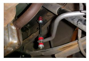
17. On the driver side of the vehicle, locate the 1/2" hole on the lower flange of the frame, in front of the axle. Raise the arms of the sway bar so they are parallel with the frame, the hole on the frame will be above the hole on the sway bar end. Assemble the end link as on the frame and sway bar as shown in the diagram on page four. Place the end link bolt in from above so the bolt head faces up and the nut is at the bottom. Hand tighten but do not torque yet.
