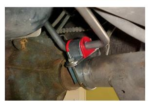
20. Tighten the end link nuts to the point where the spacer tube can still be forced to rotate on the bolt by hand, but the grommets should not be able to rotate by hand. Torque the end link bracket securely to the frame on the passenger side.
